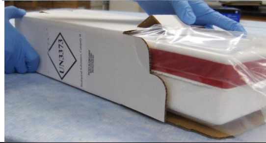
Figure S5: Kit assembly instructions shows packaging of kit according to IATA standards and assembly into a corrugated shipping box with the correct markings.
